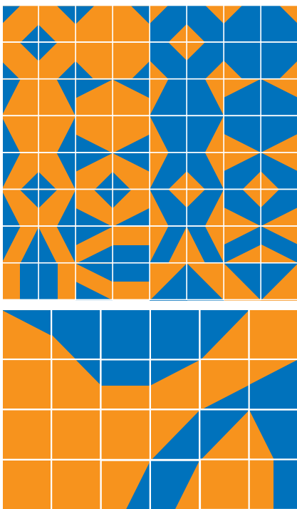
FIGURE 5 A transition tile allows edges with multiple edge types. The minimum set of tiles is larger, but the layout is much more flexible and diagonal connections are now clear.
